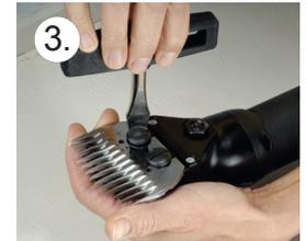
Tighten both screws just enough to hold the comb in place. (You will securely tighten the screws later.)
